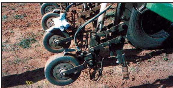
The pressurised liquid system injects Flexi-N behind the seeding tube and in front of the presswheel.
